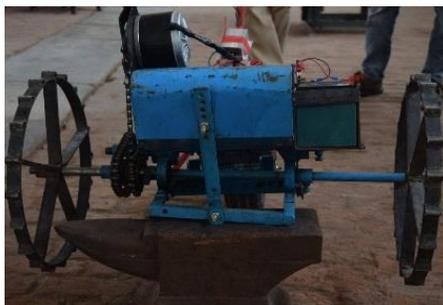
Fig. 4. Motor-operated seeder during calibration
