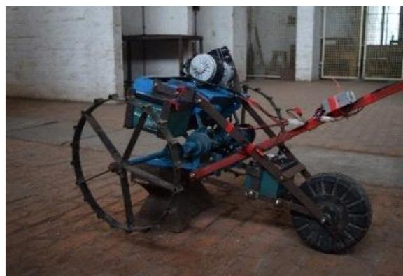
Fig. 2. Motor operated seeder
