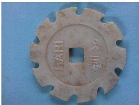
Fig. 5. Seed metering device
