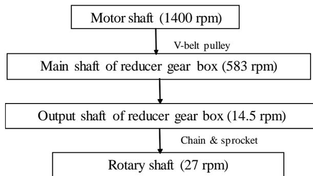
Fig. 4. Power transmission system of the turmeric polisher
