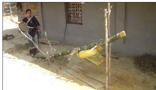
Fig. 9. Paddle-operated polishing method
